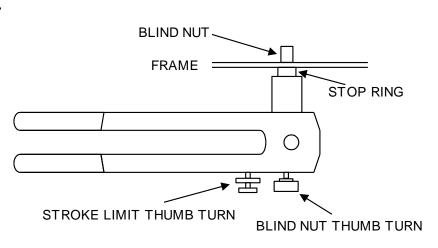
stop ring does unscrew for removal (this is part of the procedure of changing the threaded stud). It can easily become loose. You turn it counterclockwise to tighten it and clockwise to remove it.
